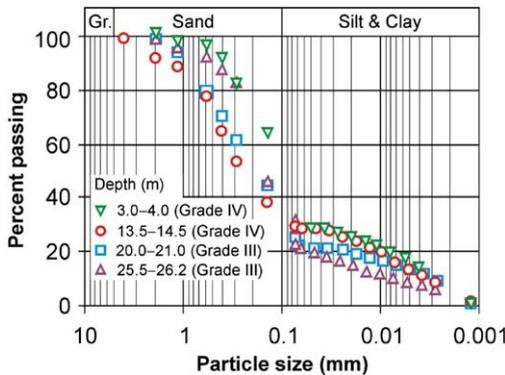
Fig. 5. Particle size distributions of residual soils at different depths from the Jurong sedimentary formation (NTU-CSE slope).
