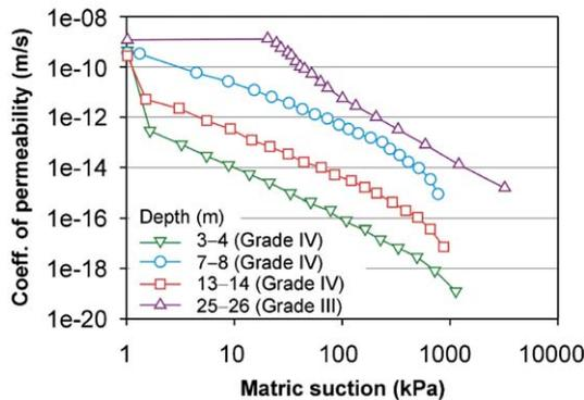
Fig. 13. Permeability functions of residual soils from different depths of the Jurong sedimentary formation (NTU-CSE slope).
