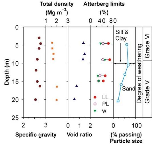
Fig. 6. Index test results of residual soils from different depths of the Bukit Timah granitic formation (Yishun slope).
