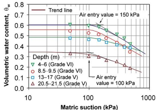
Fig. 10. Soil–water characteristic curves of residual soils from different depths of the Bukit Timah granitic formation (Yishun slope).
