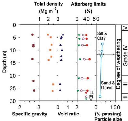
Fig. 7. Index test results of residual soils from different depths of the Jurong sedimentary formation (NTU-CSE slope).
