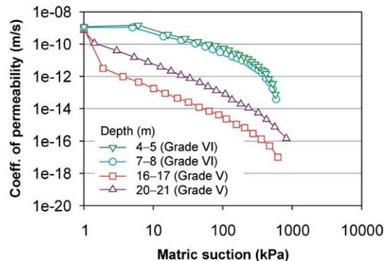
Fig. 12. Permeability functions of residual soils from different depths of the Bukit Timah granitic formation (Yishun slope).
