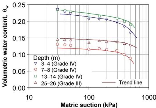
Fig. 11. Soil–water characteristic curves of residual soils from different depths of the Jurong sedimentary formation (NTU-CSE slope).
