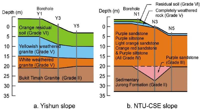
Fig. 3. Typical weathering profile of residual soil from (a) Bukit Timah granitic formation (Yishun slope); (b) Jurong sedimentary formation (NTU-CSE slope).
