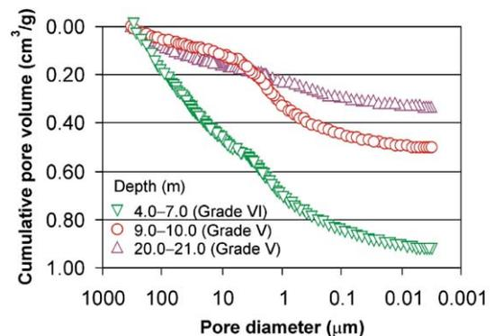
Fig. 8. Pore-size distribution of residual soils from different depth of the Bukit Timah granitic formation.
