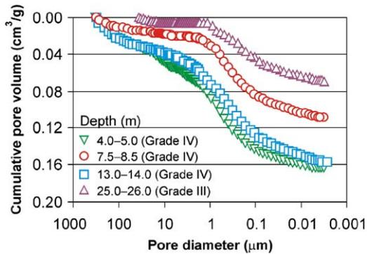
Fig. 9. Pore-size distribution of residual soils from different depth of the Jurong sedimentary formation.
