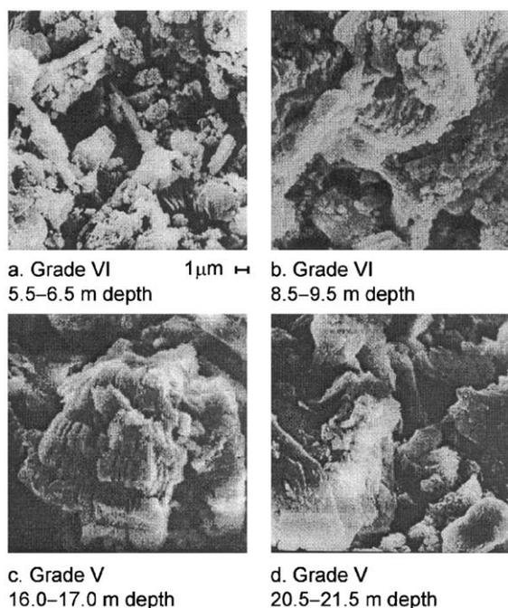
Fig. 14. SEM images at  $5000\times$  magnification of residual soils from the Bukit Timah granitic formation at depths of (a) 5.5–6.5 m; (b) 8.5–9.5 m; (c) 16–17 m; (d) 20.5–21.5 m.
