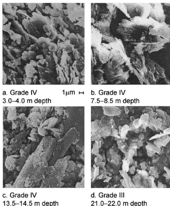
Fig. 15. SEM images at  $5000\times$  magnification of residual soils from the Jurong sedimentary formation at depths (a) 3–4 m; (b) 7.5–8.5 m; (c) 13.5–14.5 m; (d) 21–25 m.
