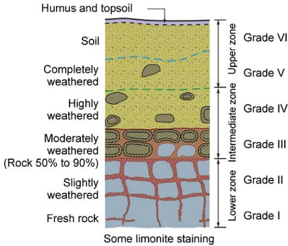
Fig. 2. Typical weathering profile of residual soils (from Little, 1969).
