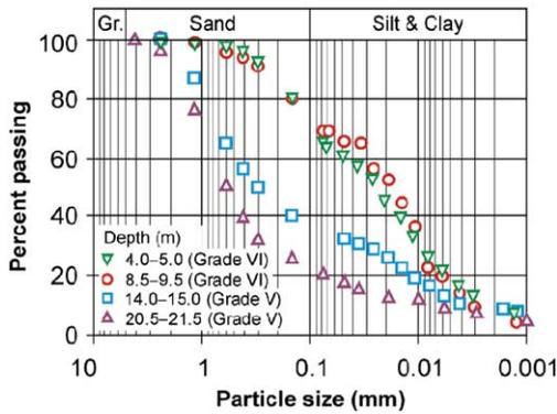
Fig. 4. Particle size distributions of residual soils at different depths from the Bukit Timah granitic formation (Yishun slope).
